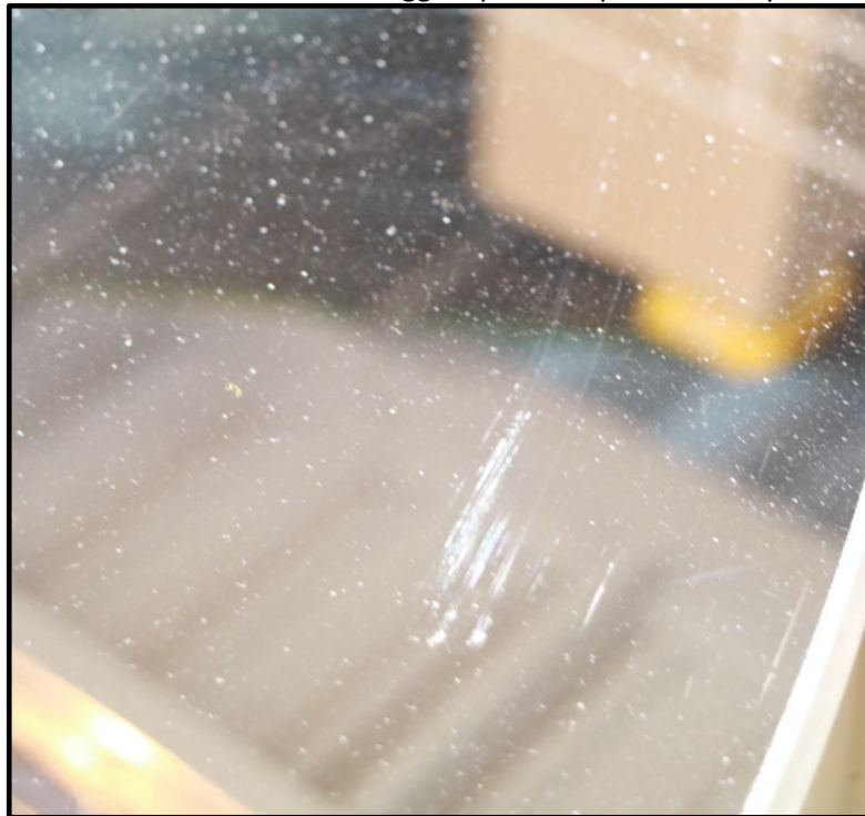
Fig 1. (above) closeup of stained, scratched area near top edge (radial extent ~5cm). First Contact polymer was applied several times to this area, reducing stain, but scratch damage remained. See also spotting: why some appear elongated is uncertain.
