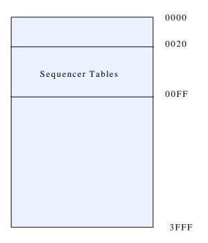
The values used to set the DAC voltages to set the bias voltages for the array are stored here along with sequences themselves which are used to produce the clocking routines to readout the array.
