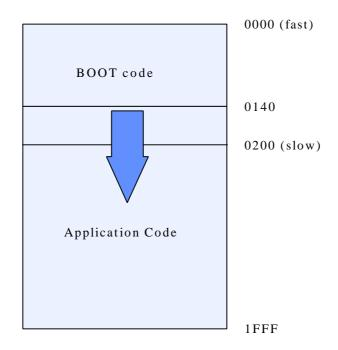
This shows the internal P memory area after the application code has been downloaded. This code overlaps both the internal fast DSP RAM and the slower external RAM. This means that it is important to ensure that the code required to run as fast as possible sits in the internal low memory area. This area is also limited so that very efficent code needs to be written to fit in here. All the sequencer routines for reading out the array are stored from P:0140 to P:01FF.
