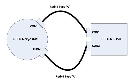
N.B. Red+4 Type 'B' cables exist but should not be used for single amp operation.
