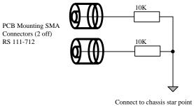
This cabling allows two channel readout of the red sensitive mosaic CCD as well as the 2EEV. It is compatible with the WHTWFC wiring so the controllers could be interchanged for spares.
