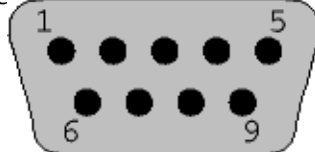
Figure 5 – SGI 9-Pin Connector
