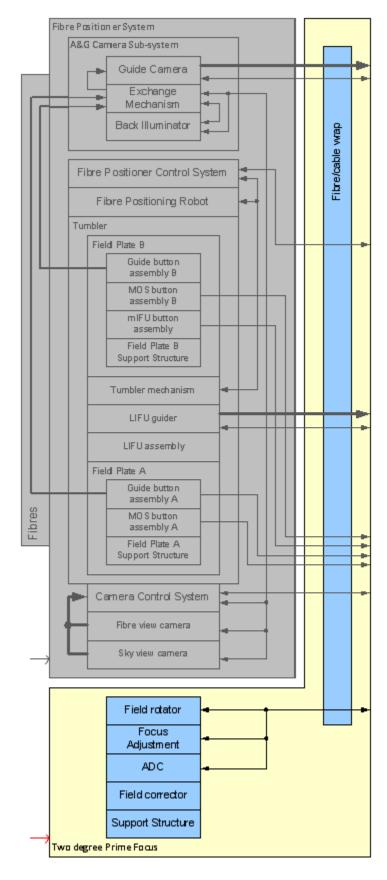
The Two-degree Prime Focus system (PRI) is composed of:
