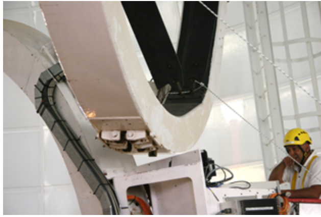
Figure 6: The ring clears a support bracket, on the fixed ring, by millimetres leaving the Head of the Mechanical Section somewhat apprehensive.
