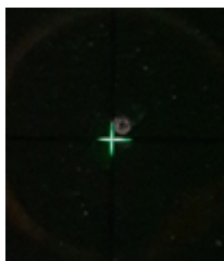
Figure 2: A collimated green beam was propagated through the crosshair of the alignment telescope, reflected off the secondary mirror and its position, with respect to a circular reference mark on the mirror, was recorded.
