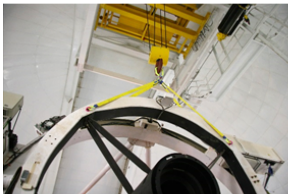
Figure 4: The flip ring is lifted using the WHT 25-T crane.
