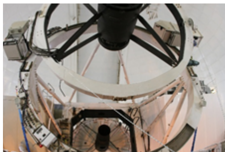
Figure 5: Images showing the moment when the flip ring was separated from the fixed ring.
