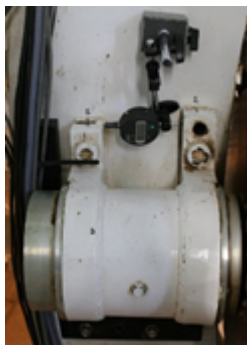
Figure 3: The left-hand bearing, with the dowel pins (only one shown in picture) removed, showed no movement of the bearing housing with respect to the outer ring. After removing the four bolts, a small movement (80µm) to the left of the bearing housing was seen. Before continuing with the process, it was confirmed that this displacement could be recovered.
