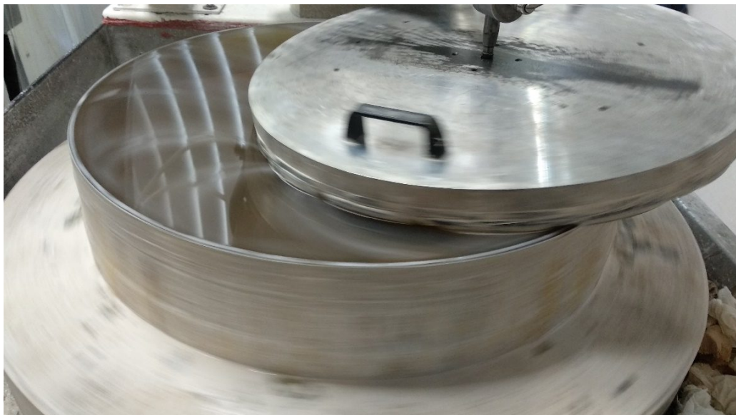
Figure 8. (a) Detail of the polishing pitch tool, 600 mm diameter. (b) Polishing process.
