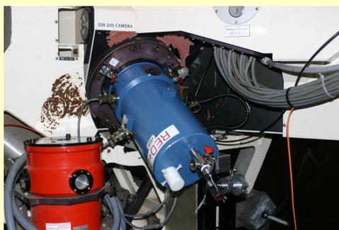
The recently commissioned 2k x 4k pixel Deep depletion low fringing device from E2V mounted on the 235 mm camera of IDS. The camera gives 3-4e noise, dark current <math>8e/hour</math> and linearity <math><1\%</math> up to 60kADUs
