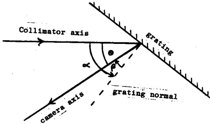
**Figure 3** Geometry of the grating.
