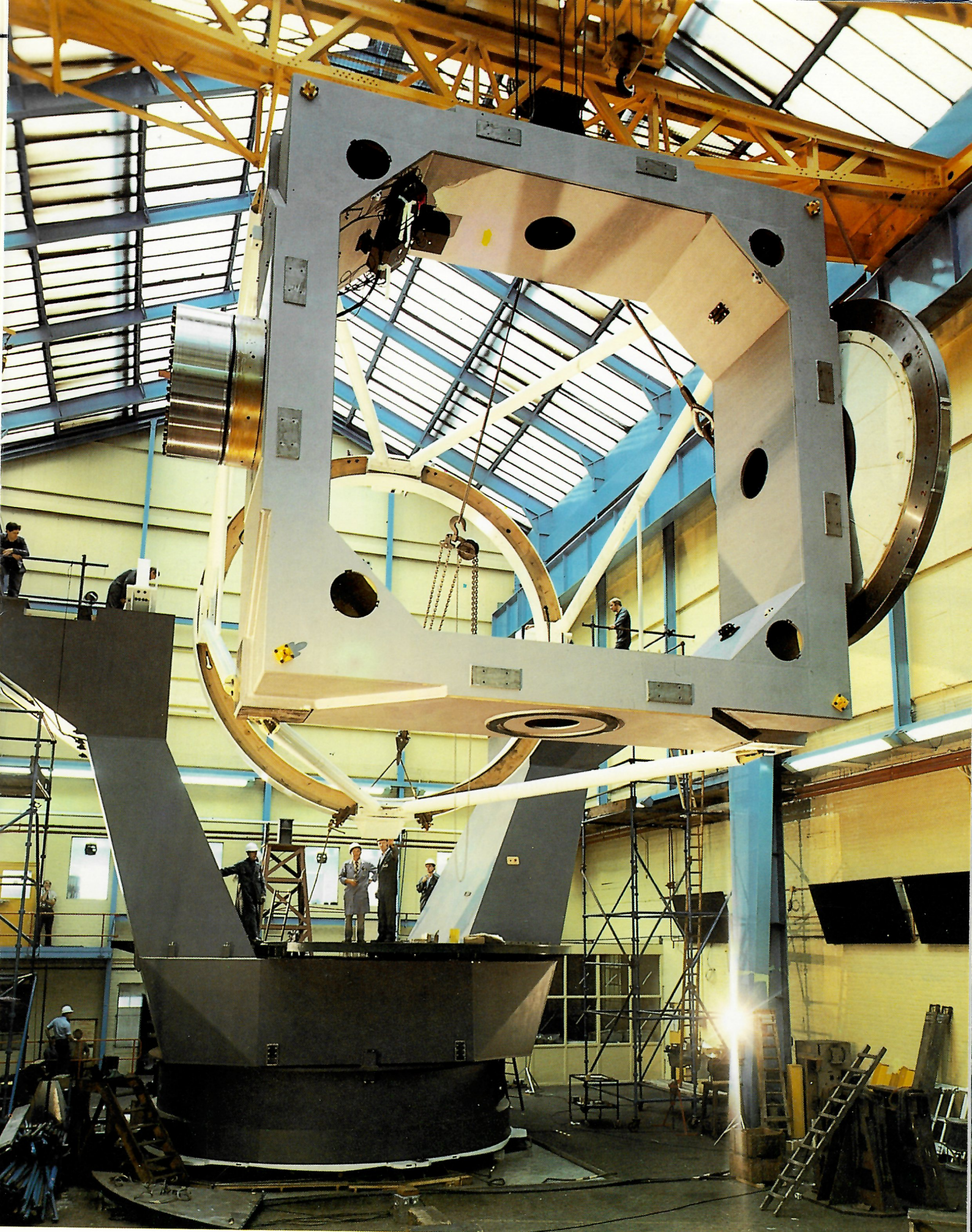
THE 4.2 METRE WILLIAM HERSCHEL TELESCOPE during assembly by Grubb-Parsons in Newcastle-upon-Tyne.
