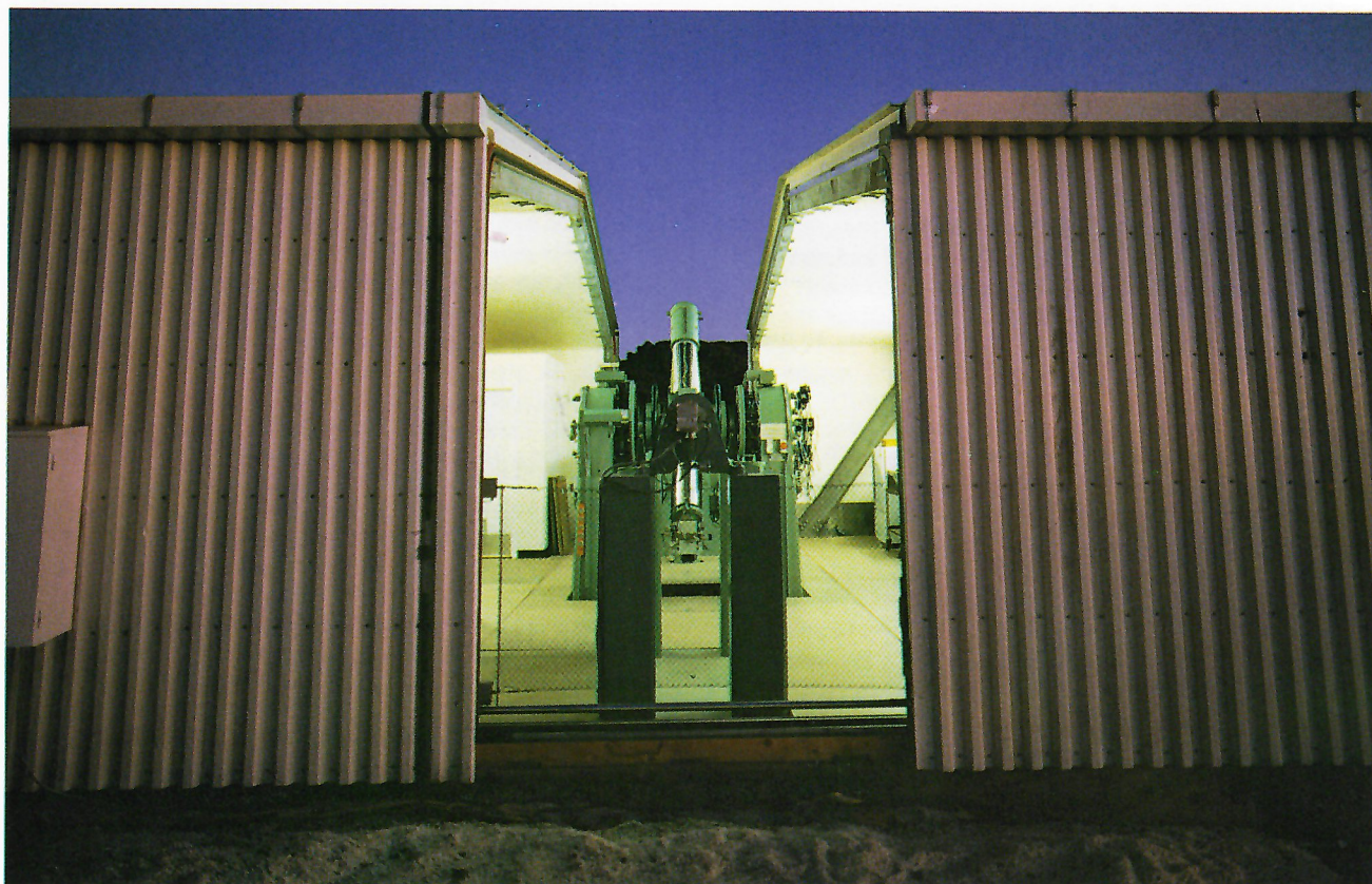
Fig. 2 The Carlsberg Automatic Meridian Circle moves in a north-south plane, looking through a slit which opens in a roll-off building to the stars which transit above the instrument.
