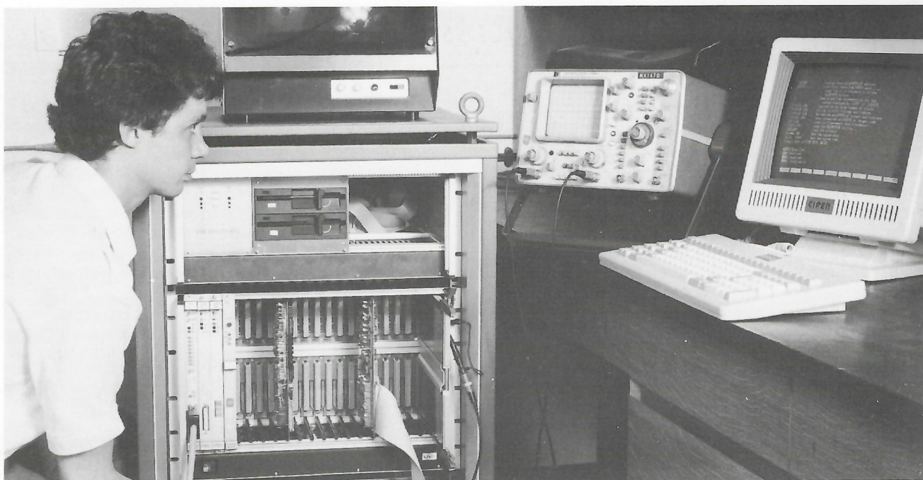
Fig. 1 VME microprocessor system under test in the RGO workshops.
