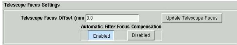
*The Automatic Telescope Focus Adjustment Panel*
