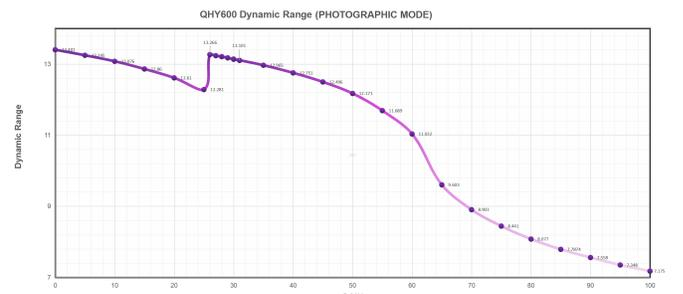
**Readout Mode #1 (High Gain Mode).** In this mode, the QHY600 switches from Low Gain to High Gain between gain settings of 55 and 56. Gain 0-55 uses LGC and Gain 55-100 used HGC.
