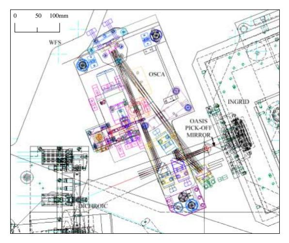
Figure 1.1 OSCA unit relative to the other components on the NAOMI optical table in GHRIL.
