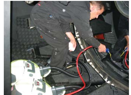
Vapour cleaning (left) and drying (right) INT primary mirror.
