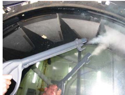
Vapour cleaning (left) and drying (right) INT primary mirror.
