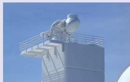
From top to bottom: one of the NSST mirror blanks in the aluminising area at the WHT, pad gluing in the rear of one of the blanks and the two mirrors assembled on top of the NSST tower.
