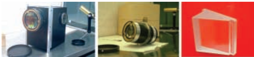
From left to right: Figure 2. Collimator. Figure 3. Camera. Figure 4. Corning 9754 Grism.
