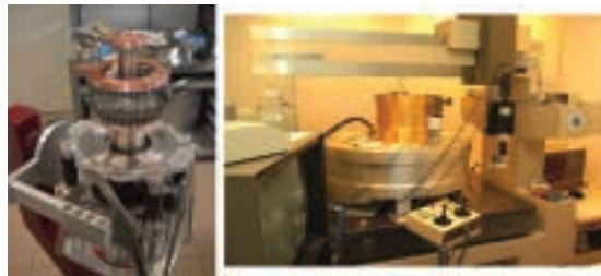
From left to right: Figure 5. Slit wheel. Figure 6. Pupil wheel. Figure 7. Camera wheel integrated in the test cryostat (dummy on camera position).
