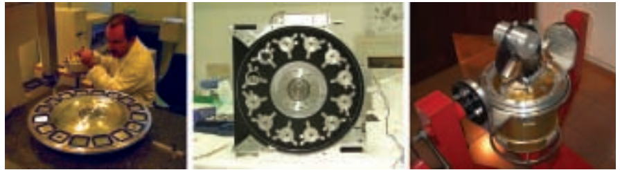
From left to right: Figure 5. Slit wheel. Figure 6. Pupil wheel. Figure 7. Camera wheel integrated in the test cryostat (dummy on camera position).
