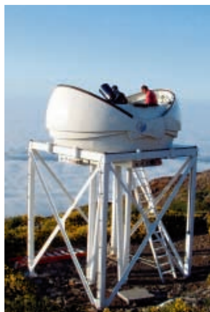
Figure 3. RoboDIMM tower, dome and telescope.
