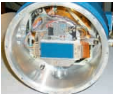
Figure 2. A photo of one of the ING cameras (with a test chip mounted) complete and awaiting the delivery of the first red CCD.
