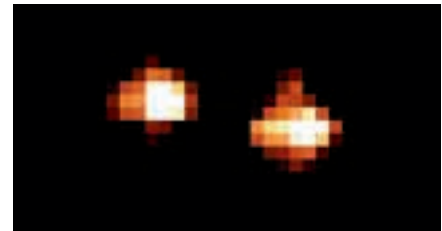
Figure 1. This 0.5-arcsec double star, R=11 , was selected from the Palomar Sky Survey (on which it is unresolved) as the guide star for NAOMI observations of a nearby QSO. The wavefront sensor took this double image in its stride, and the delivered FWHM on the above 30-sec H-band exposure is 0.16 arcsec.
