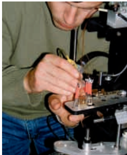
Figure 3 (left). Alignment of fibres into micro-lens finger holder. Figure 4 (top right). Fingers mounted onto the facet block. Figure 5 (bottom right). The Small Fibre Module at WHT prime focus.
