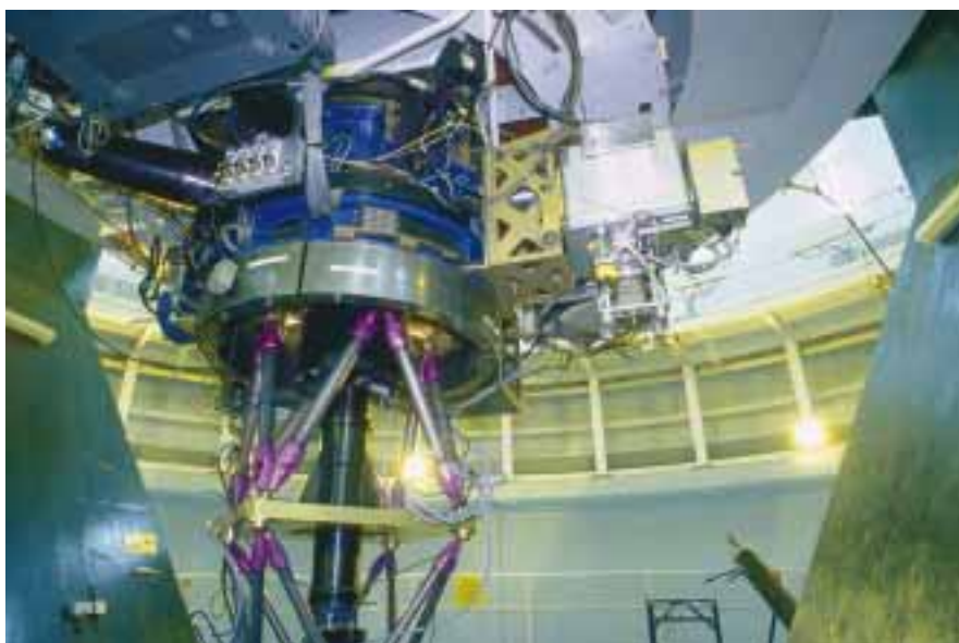
Figure 3. INGRID mounted on one of the WHT folded Cassegrain foci (top right). The instrument on the Cassegrain focus is SAURON. Picture credit: Rainer Girmstein.
