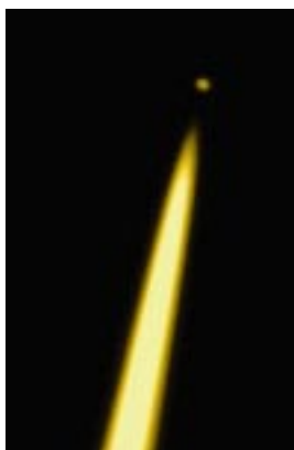
Figure 3. A pseudocolour image of the laser scattering taken with a small telescope 3m away from the laser launch. The small spot at the top is the sodium laser beacon.
