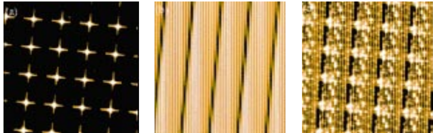
Figure 4. Examples of various SAURON calibration measurements, taken during commissioning. Each panel shows only a small part of the entire CCD frame so that details can be seen. a) Micropupil image taken with the grism out. Each dot is the diffraction pattern from one square lenslet. b) Continuum image using the tungsten lamp. c) Neon arc.
