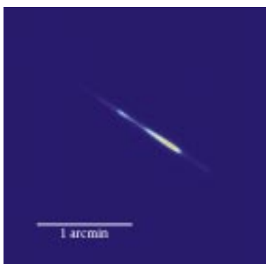
Figure 4. A pseudocolour image of the resonant backscatter from the sodium layer as viewed from the JKT at midnight 22 September 1999.
