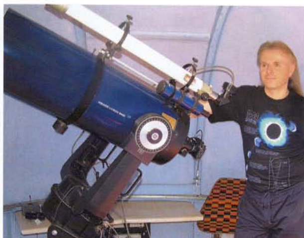
Nik Szymanek in his Essex-based back-garden observatory. The telescope is a 10-inch Meade LX200. Mounted on top is a Vixen 60 mm refractor used for autoguiding with an SBIG ST-4. Image: Nik Szymanek.
