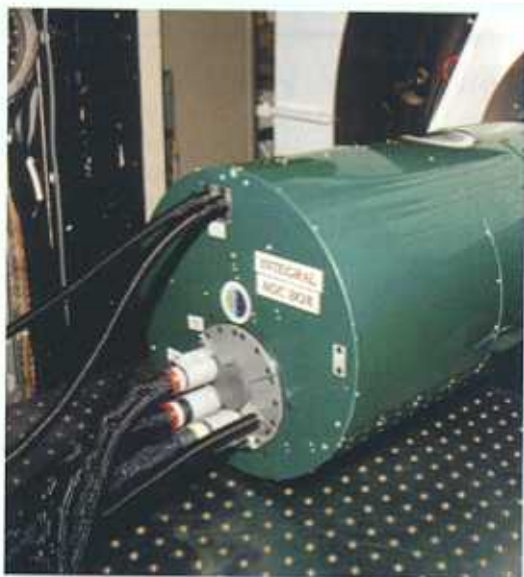
The integral fibre optic unit on the WHT. Photo Courtesy of the Integral Team, Isaac Newton Group of Telescopes, La Palma.
