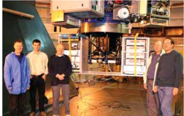
Figure 39. The PLANETPOL instrument mounted in the Cassegrain focus of the WHT, together with the team of scientists.
