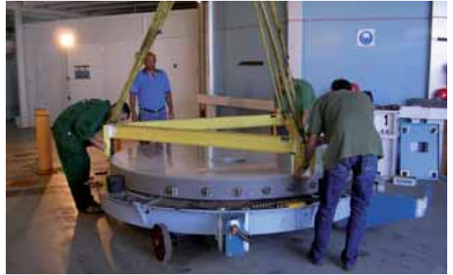
Figure 42. Lifting of primary mirror of the Nordic Optical Telescope in preparation for aluminizing.
