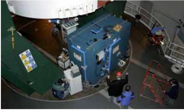
Figure 38. The CIRPASS IR spectrograph (blue cabinet) being positioned on the moving platform at the base of the WHT. Light from the Cassegrain focus is fed through a large bundle of fibres to the spectrograph.
