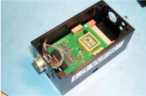
Figure 34. The Low-Light-Level CCD that will be deployed as wavefront sensor in the AO system. The actual CCD chip is the tiny black square in the yellow enclosure.
