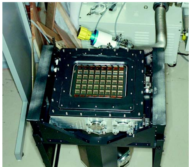
Figure 13. Mosaic CCD Camera II (MCCDII). Forty CCDs are seen aligned in a 5 \times 8 array. A liquid nitrogen tank is attached backside of the Dewar to cool the CCDs down to appropriate temperature.
