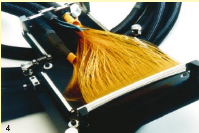
4.- INTEGRAL fibre bundles mounted in a WYFFOS slit unit.
