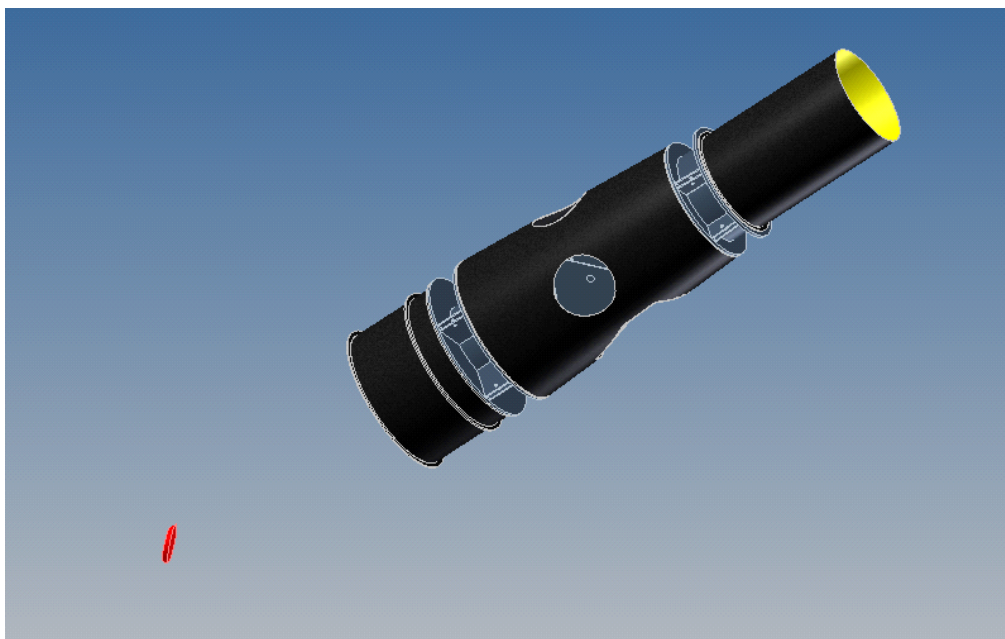
Fig 2. Acam fold mirror (red) with Nasmyth turret assembly. Note inside of sky fog baffle has been highlighted in yellow for clarity.
