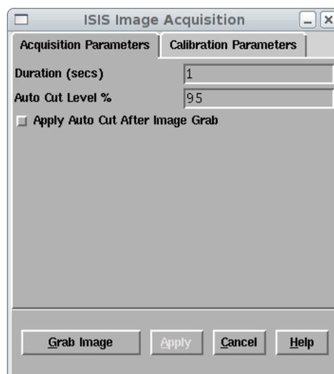
The **Duration Field** will allow the user to specify the length of the integration when acquiring the acquisition image and will be expressed in seconds as a real number.
