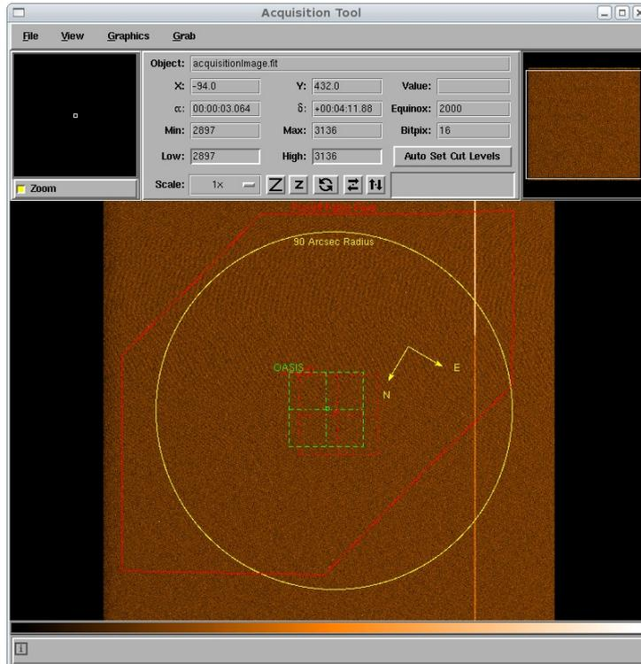
Illustration 1 Main application window showing NAOMI/INGRID acquisition image and all overlays
