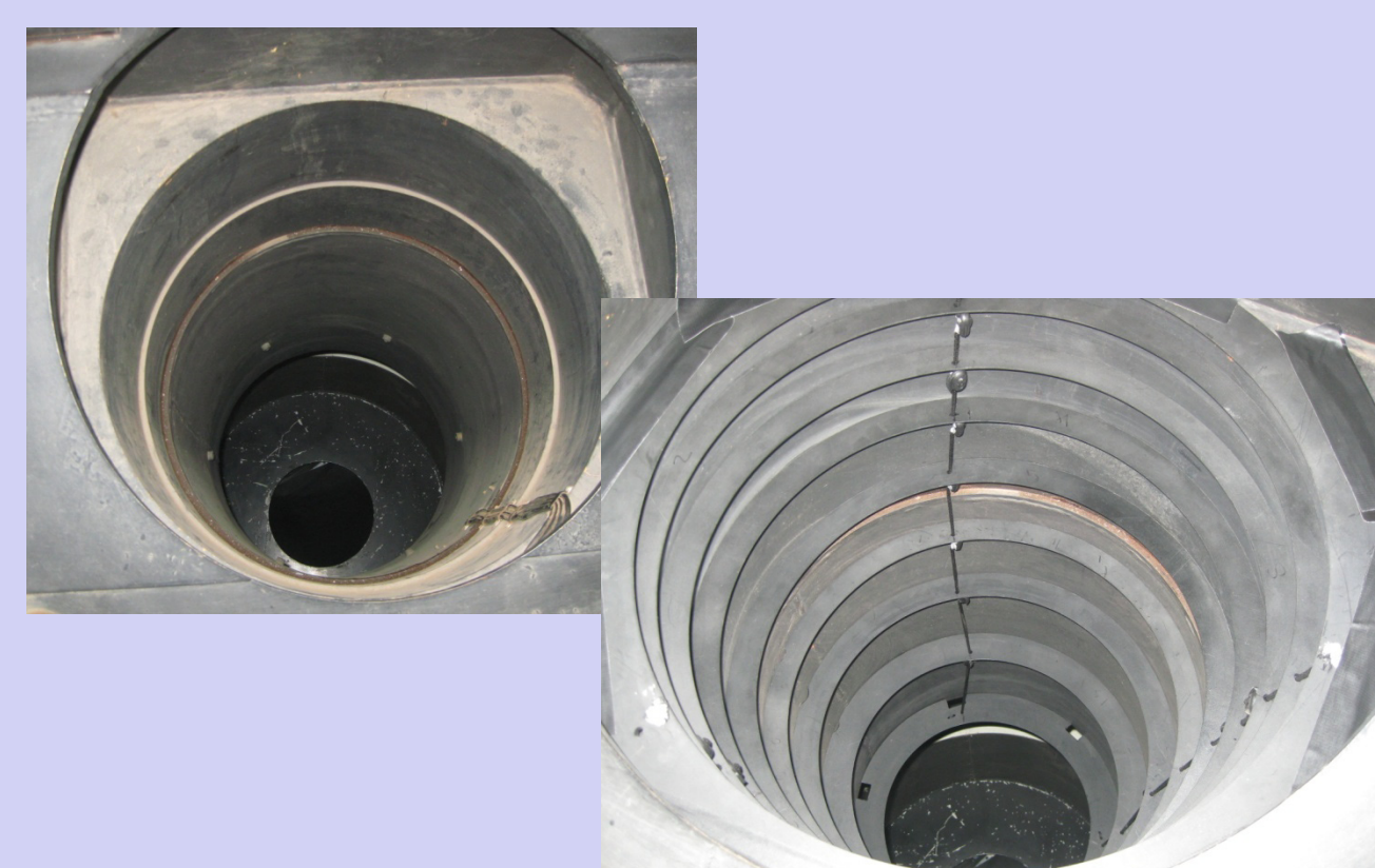
Fig. 4. ACAM images taken near the moon suffer from scattered moonlight (above left). A 'Chinese lantern' of plate baffles was installed in the WHT's below-Nasmyth turret in November 2011 (above right, before and after installation), and has reduced the intensity of the scattered light by \sim 70\% . Investigations continue.
