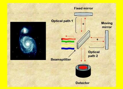
The Inverse Fourier Transform changes the Optical Path Difference into frequency (inverse of wavelength).
