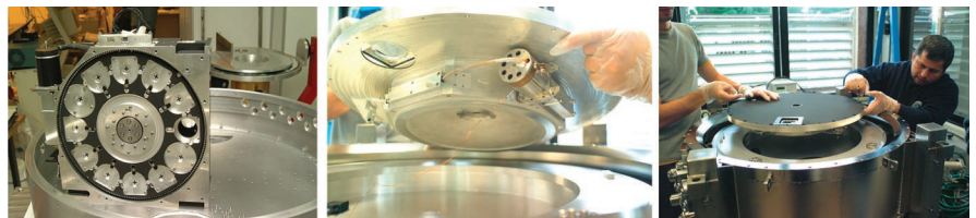
From left to right: Figure 10. Main central wheel module (filter wheel side) pre-integrated on LIRIS. Figure 11. Bottom view of the slit wheel mechanism. Figure 12. Pre-integration of the slit wheel on the LIRIS optical bench.
