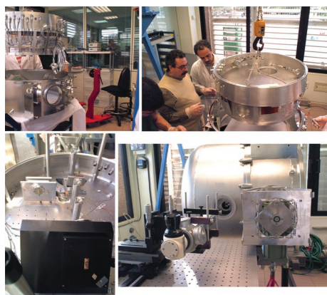
From top to bottom: Figures 15 and 16. Positioning the optical bench on the trusses in the vacuum tank central ring (cables provisionally fixed for this cycle). Figures 17 and 18. Optical bench with the collimator and reticules placed in specific positions to check their behaviour during the first cycle (these reticules were visible at all time through a very useful cryostat auxiliary window, see Figure 18). A simulation of the detector module was placed outside the beam line to test the detector thermal control system.
