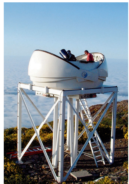
Figure 3. RoboDIMM tower, dome and telescope.
