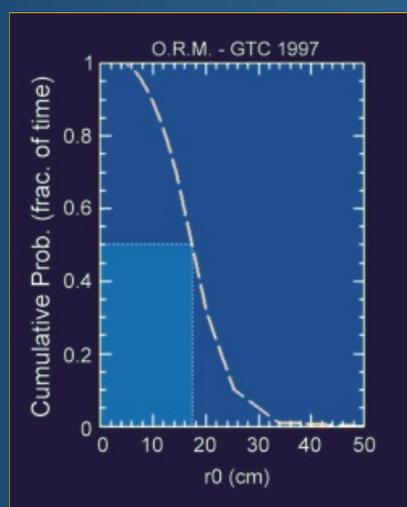
Cummulative frequency of seeing measurements (55545 data) at the GTC site. For 50% of all cases, the seeing value is smaller than 0.58arcsec ( $r_0$  larger than 17.4cm).
