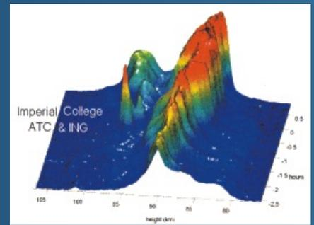
*The Sodium profile variation at ORM. Data from one half night (22nd September 1999). The figure shows a large, slow variation in the shape and total area of the sodium profile, as well as a sporadic event of high sodium concentration, lasting a about 15 minutes (from MNRAS, 318, 139 (2000); see also [http://op.ph.ic.ac.uk/jkt\\_lgs/](http://op.ph.ic.ac.uk/jkt_lgs/)).*
