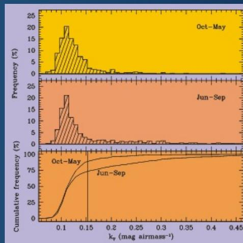
Frequency of extinction over the ORM during winter (top) and summer period (centre). In both cases the modal value is found at 0.11 mag/airmass. Their corresponding cumulative frequencies are also shown (bottom). The vertical line indicates the extinction coefficient limit for dusty nights,  $k_v \geq 0.153$  mag/airmass (PASP 2001).
