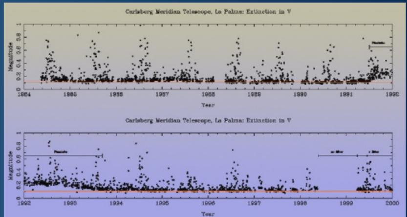
From observations of about 50 photometric standards, the Carlsberg Meridian Telescope provided nightly values of atmospheric extinction in V for ORM. The data is split up into yearly files going back as far as 1984. The most recent file is that for 2000 January - May. From the end of 1999 March this differs from previous years as it is derived from the new CCD camera which works in the Sloan r' band.
