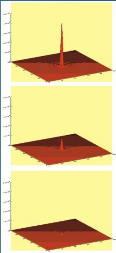
Images that would be obtained using an adaptive optics system ( $\lambda = 1.65 \mu\text{m}$ ) with a deformable mirror with 100 actuators on a GTC-type telescope for three different values of seeing: 0.5 arcsec, 1.0 arcsec and 1.5 arcsec. The plate-scale is the same for all three images.
