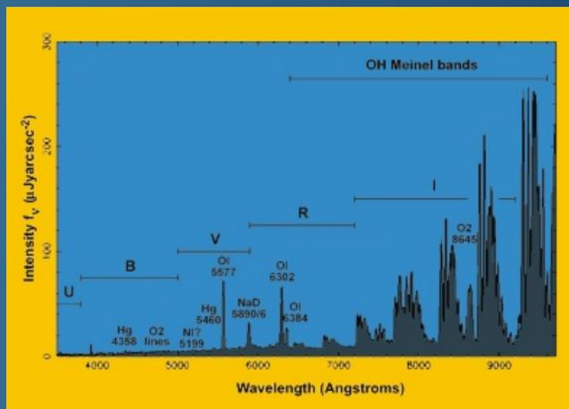
*Typical spectrum of the La Palma sky on a moonless night. Most of the distinctive features of the night-sky spectrum are due to airglow. The NaD emission at 5890/6 Å is partly due to street lighting, while the mercury emission at 4358, 5461 Å is wholly so. With the exception of the 8445-Å O<sub>2</sub> line, the features dominating the spectrum redward of 6500 Å are the Meinel rotation-vibration bands of OH. (New Astronomy Reviews, 42, 503 (1998)).*
