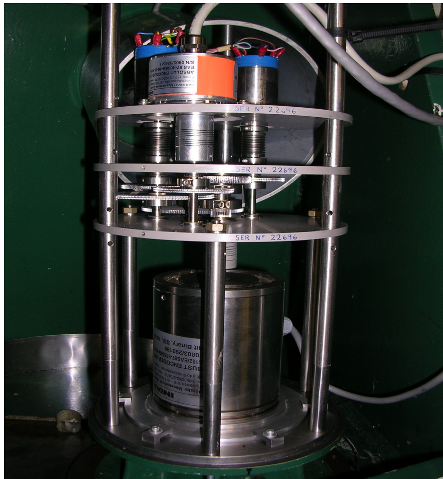
Picture 2: Assembly of the Az absolute encoders + synchros
