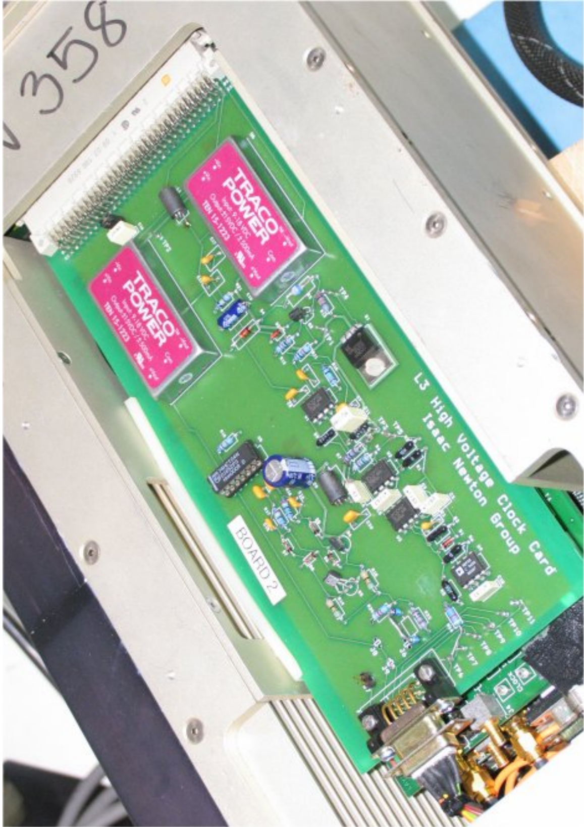
ING HV board mounted in an SDSU II controller
