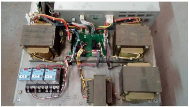
Three relays K1,K2 and K3 have been installed on a DIN rail next to the control card and wiring interconnection (Ref: 8135167G001).
