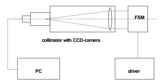
The FSM will be placed in front of a collimator. The collimator has an illumination unit and a CCD-camera system. The FSM will be controlled with voltages, which become smaller. The smallest voltage skip is 0.24mV (10V, 12 bit).
