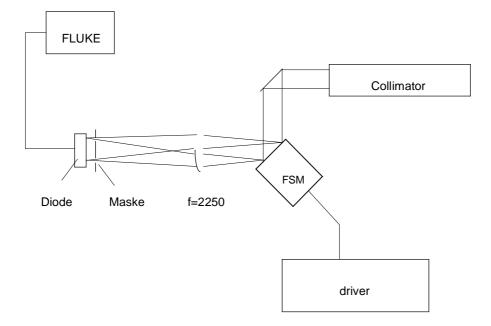
In front of the large-size diode a mask with a double slit will be placed. The distance of the slits is  $s = 2*2250*tan(103.1arcsec)=2250 \ \mu m$ . Light incidence on the diode only takes place, if the FSM generates a beam deviation of 103.1 arcsec (= 500 \ \mu rad). The signal will be recorded on an oscilloscope (FLUKE).
