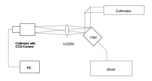
The axes x and y of the FSM will adjusted successively in 10 positions each. The spot positions will be measured and recorded with a collimator with CCD-camerasystem The rectangularity will be calculated from the positional field by means of an adjustment method.
