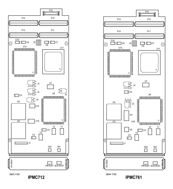
Figure 1-1. IPMC Component Layout
