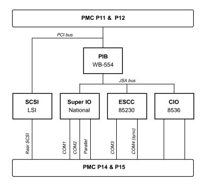
Figure 1-2. IPMC712 Functional Block Diagram
