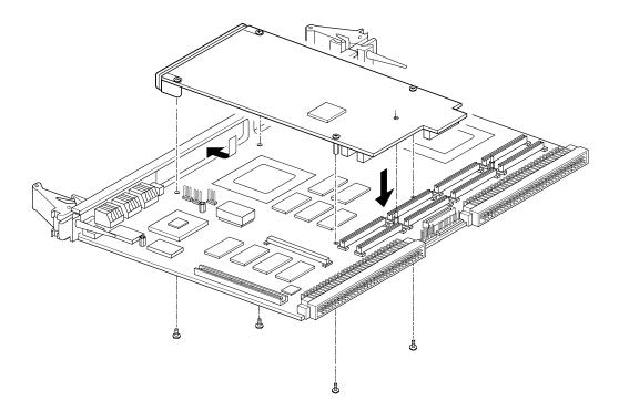
Figure 2-1. IPMC Installation
