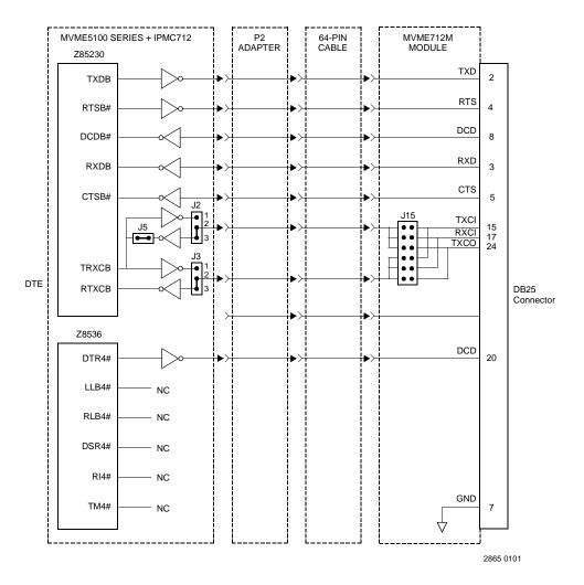
Figure 1-3. IPMC712 Serial Port 4 Clock Configuration
