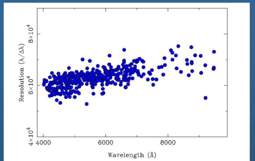
CAFE: Wavelength resolution derived from the estimation of the FWHM of the identified ARC emission lines in the dispersion axis.
