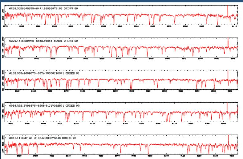
Detail of a few orders of the extracted spectra of HR4728. The actual pipeline of CAFE has been foreseen to allow the observer to make a quick&dirty reduction, visualize the data, and estimate the S/N of the data acquired at the telescope
