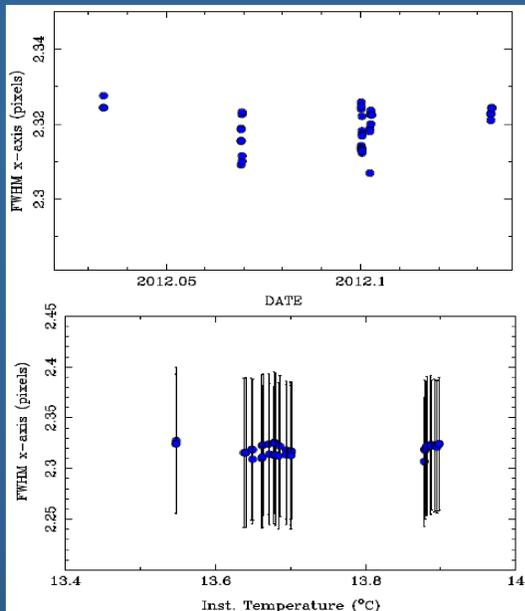
Stability of the spectral resolution. Upper panel shows the distribution of the average FWHM of the ARC emission lines along the dispersion axis for the different ARC frames. Right panel shows a similar distribution along the internal temperature of the instrument, measured with four temp. sensors.
