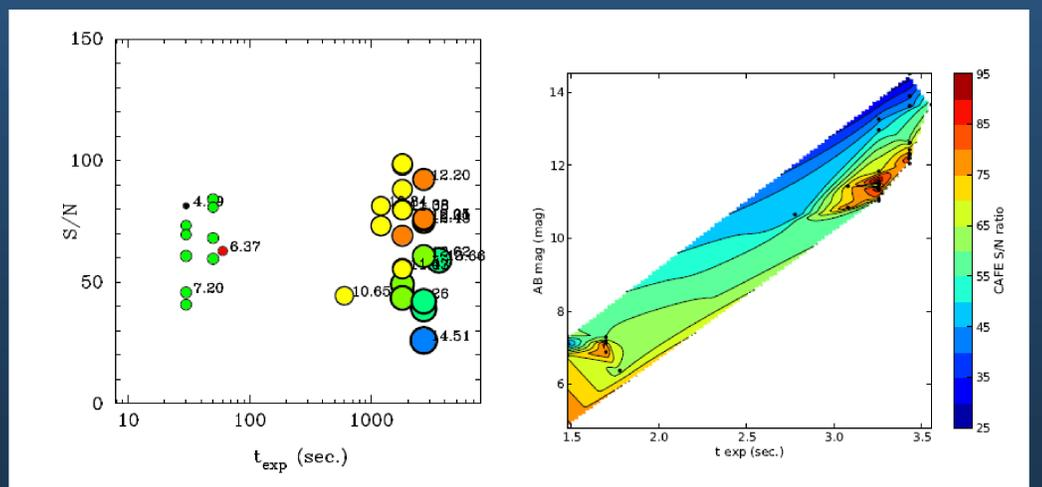
CAFE: Results from the analysis of the S/N. Left panel shows the distribution of the S/N along the exposure time, for the different observed objects. Color/size of the plotted symbols indicate the brightness of the considered object. Right panel shows the S/N distribution as a function of the brightness and the exposure time.
