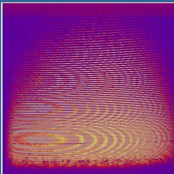
Raw data of the first science frame taken with CAFE, on the star HR4728. The orders are displayed from red, at the bottom, to blue, at the top. For each order, the wavelength range runs from blue, at the left, to red, at the right.
