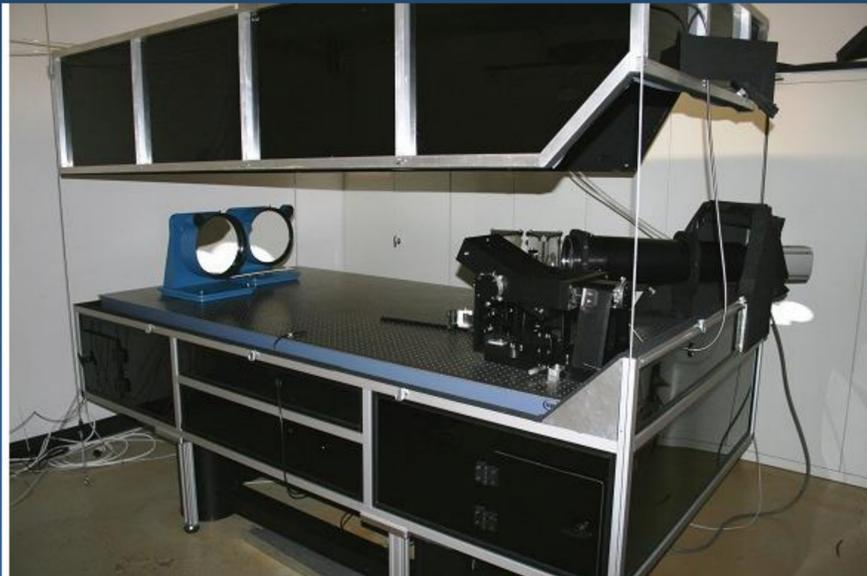
The figure shows a view of an CAFE spectrograph with the cabinet opened. The internal optical elements can be watched on the optical bench. The upper size is as straight as a die to avoid any small apertures that can break the thermal isolation. Because of that, the upper part has to be lifted up with the help of a tackle.
