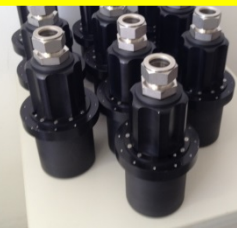
Fiber positioners "Cobra"
