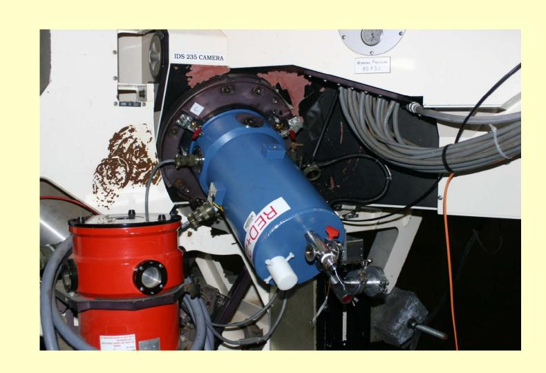
The recently commissioned 2k x 4k pixel Deep depletion low fringing device from E2V mounted on the 235 mm camera of IDS. The camera gives 3-4e noise, dark current <8e/hour and linearity <1% up to 60kADUs
