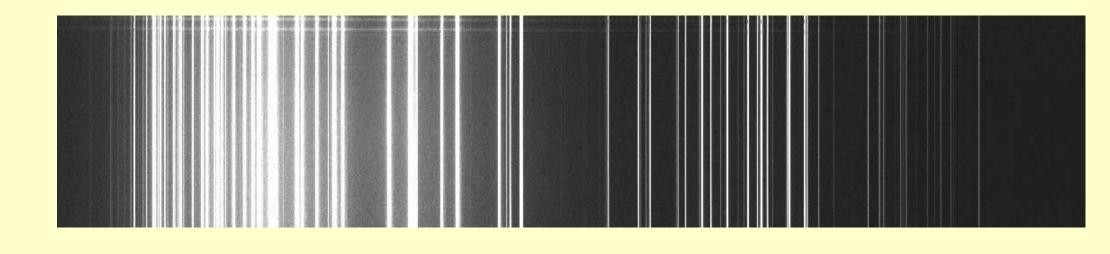
Reduced RED+2 image of CuNe arc spectrum, taken with R300V gratings, central wavelength 5520A.
