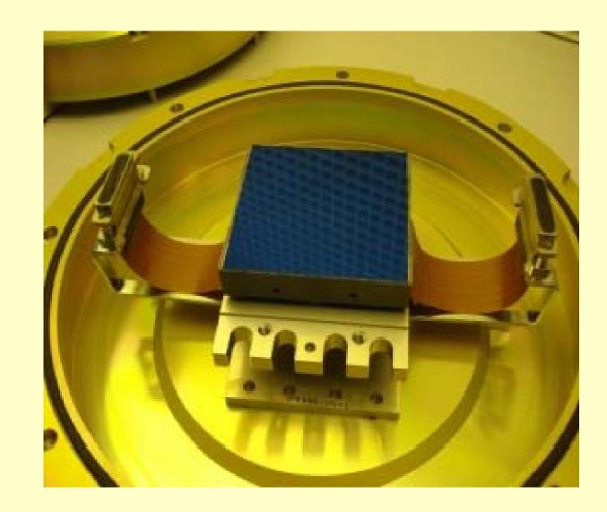
An E2V CCD231 4k by 4k pixel low fringing device has recently been received and is expected to be commissioned on WYFFOS during 2012
