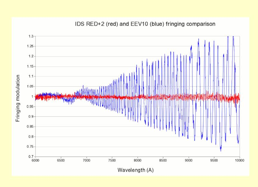
IDS RED+2 fringing plot (red) compared with that of the IDS EEV10 camera (blue), both obtained from white lamp flats taken with R300V gratings. RED+2 shows very low fringing (~ 1% in the red rising to 2% at 1000 nm) while EEV10 has severe fringing (between 3% at 700 nm and 30% at 1000 nm).
