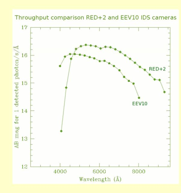
IDS throughput comparison between the former EEV10 and the new RED+2 CCD, showing the greater sensitivity of the latter in the red.
