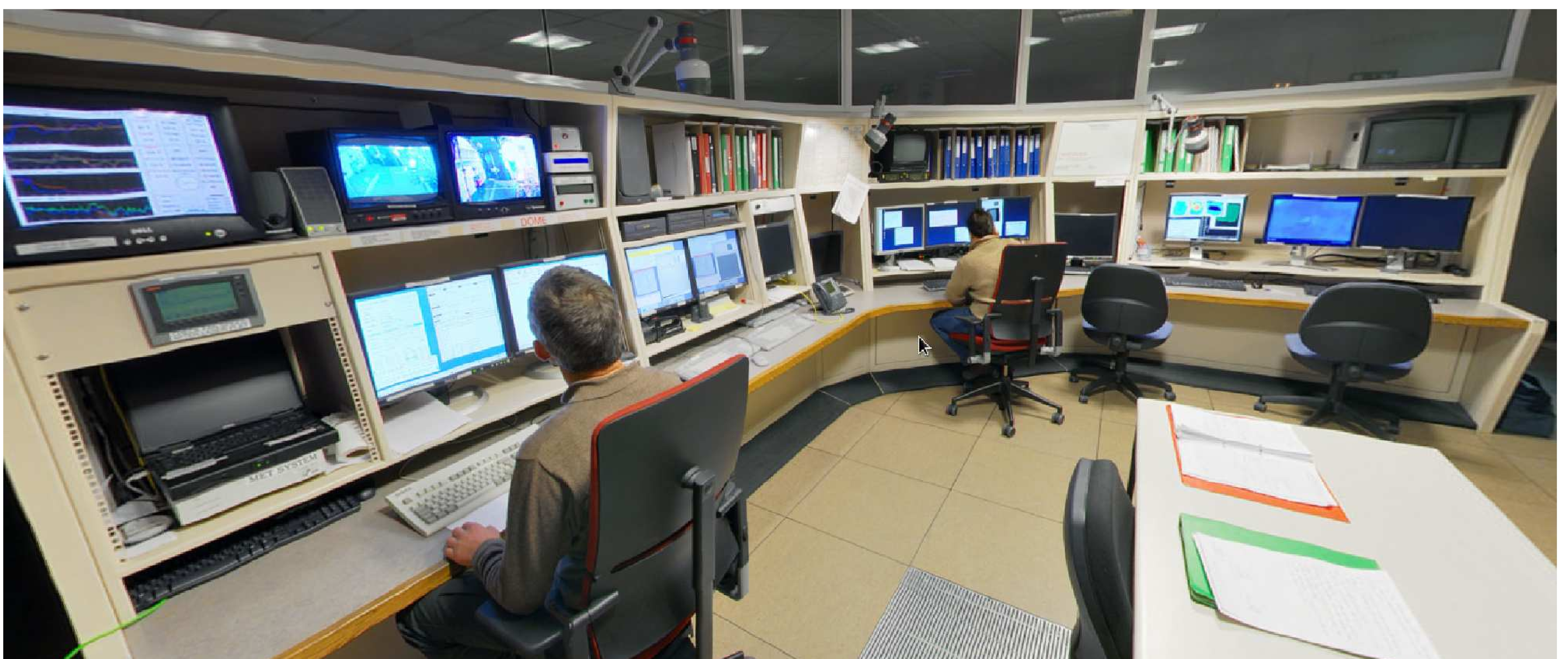
Figure 4: Control room at William Herschel Telescope. Leftmost four monitors are for Observing Support Assistant, screen for webcam, three in the middle for observer and two rightmost ones are for adaptive optics. Also seen are the screens used for data reductions.
