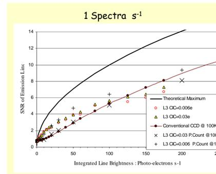
The pixel rate now needs to be 1MPixs<sup>-1</sup> to give 10 spectra s<sup>-1</sup>. A conventional CCD is capable of 5e- noise at this rate. The advantage of using L3 now becomes clearer.
