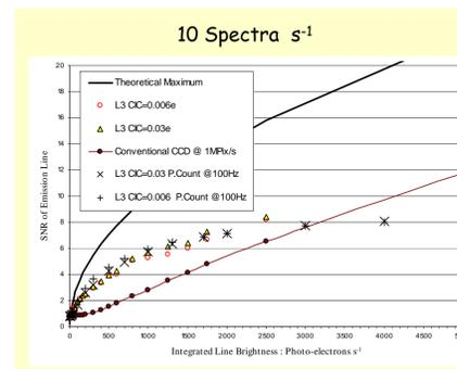
The pixel rate now needs to be 10MPixs<sup>-1</sup> to give 100 spectra s<sup>-1</sup>. A conventional CCD is capable of 20e- noise at this rate. L3 now the obvious choice.
