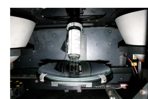
ThAr lamp and special reflector installed in the calibration unit between other two conventional lamp reflectors.
