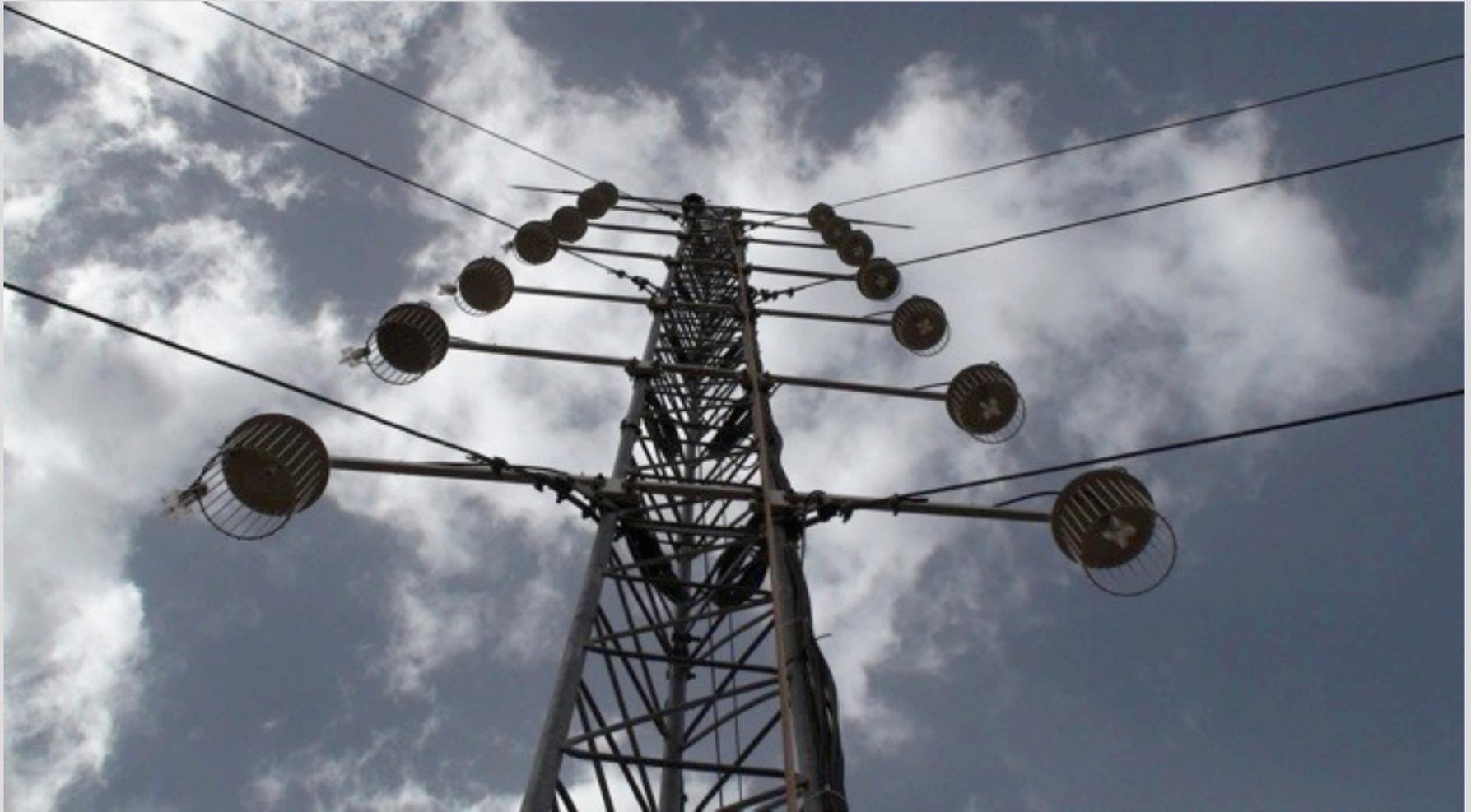
Microthermal measurements are used to determine the contribution of ground level turbulence to the astronomical seeing.
