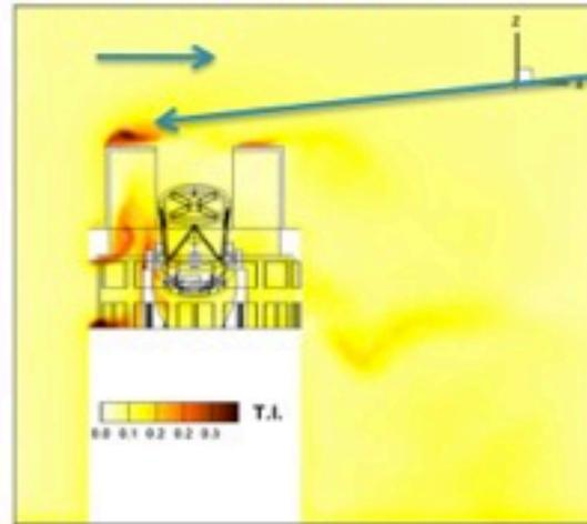
A turbulent patch is developing on the upstream side, and is likely to move over the shutter any time
