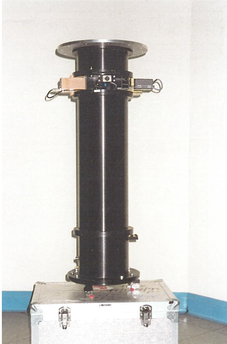
Figure I: Shack-Hartmann JKT f/15 Cassegrain configuration.
