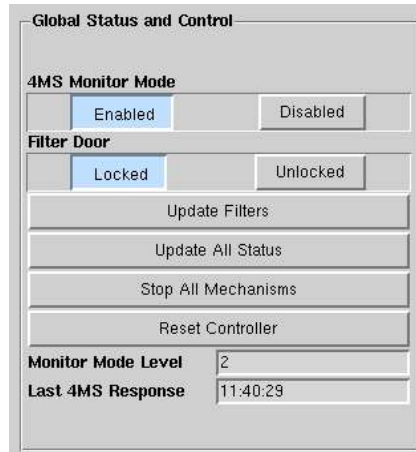
Illustration 2 Global Status and Control Panel
