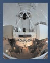
secondary mirror, made of Zerodur, 1.0 m in diameter, directs the light through a central hole in the primary mirror to the main instrumentation mounted at the Cassegrain focus beneath the primary mirror cell.
