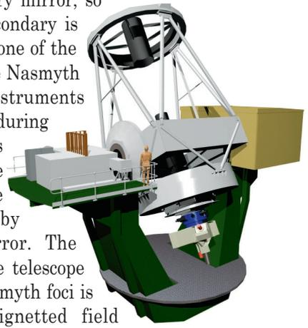
The WHT mounting is of alt-azimuth design, which requires a computer to calculate 20 times per second the motions needed in altitude and azimuth to track an object on the sky. The telescope weighs about 200 tonnes and floats on a layer of oil
