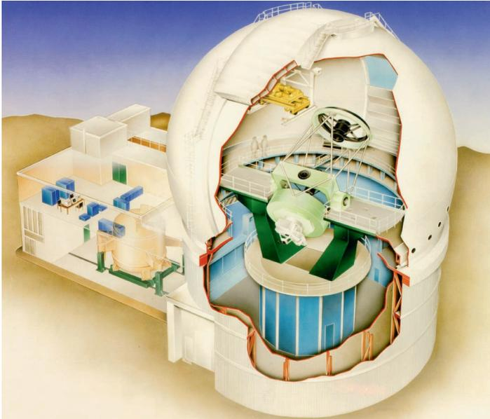
The focus of the uncorrected primary mirror incorporates a three element correcting lens to give an unvignetted field of 40 arcminute diameter. The effective focal ratio of the primary mirror with corrector is  $f/2.8$ .
