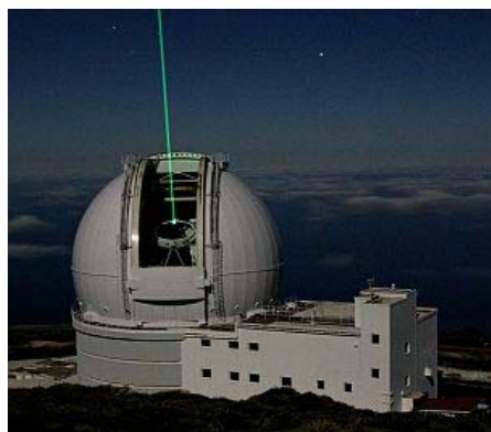
Caption: The Ground-Layer Adaptive Optics system in use at the William Herschel Telescope. Credit: Javier Méndez.
